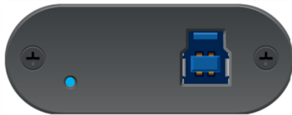
A flashing blue LED means USB 3.0
