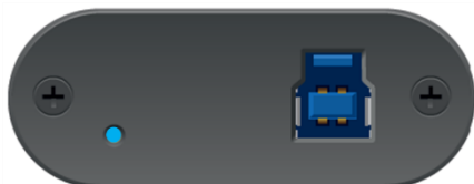
A flashing blue LED means USB 3.0
